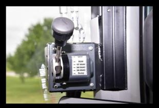
The Loader Railcar Mover package consists of Friction Drive Hi-Rail Gear, Train Air Brake system, Rear Weight Transfer Coupler and Dual Train Horns.
